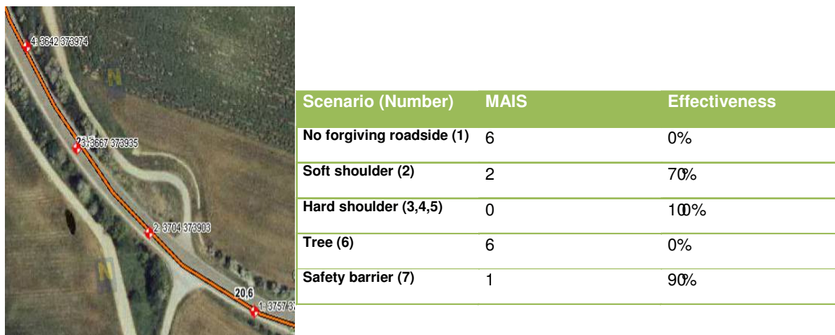
Figure 46: Example of results from the analysis of the effectiveness of having soft (unpaved) and hard (paved) shoulders in high risk bends
