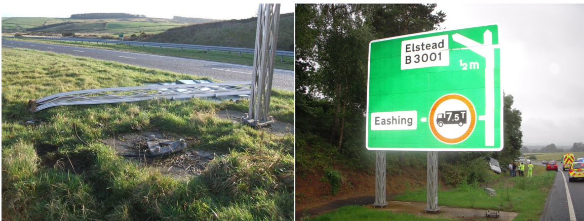
Figure 39: A 'passively safe' sign support after being hit by a passenger car [58]
