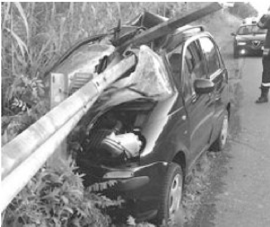
Figure 3: Head on collision with an unprotected terminal [8]
